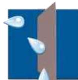
**GreenTex JGT** is designed to perform drainage functions within its own thickness. It facilitates the lateral evacuation of excess water off the construction by draining the water along its plane. **GreenTex JGT** possesses a high degree of transmissivity and is capable of holding water to about 5 times its own weight. This ensures an ongoing drainage of water, thus preventing water accumulation at the sub grade level.
